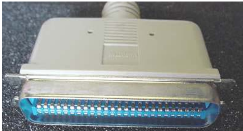
50-pins Centronics SCSI kobling
